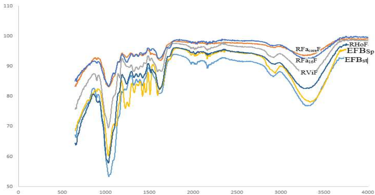
Figure 1. FT-IR spectra for the fibres.
